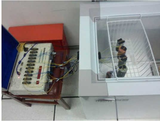
图 1 连接应变仪后的岩样 Fig.1 Samples connected with strain meter
