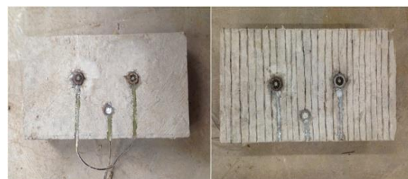
图 4 传感器安装图 Fig.4 Picture of sensor installation
