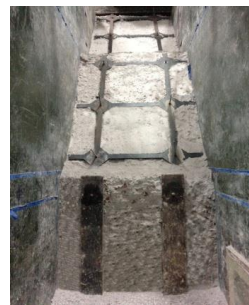
图 11 施工完成后的模型边坡 Fig.11 The model slope after construction
