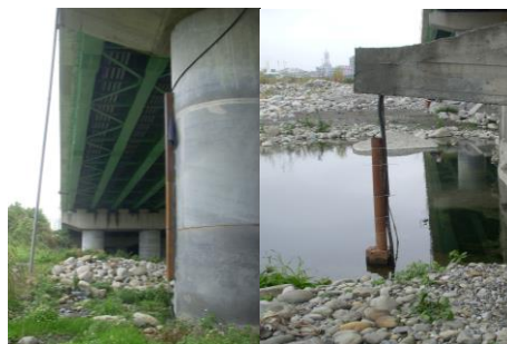
图 11 沉水式水压计建置完成图(P3/P7) Fig.11 Finished construction of sunk piezometer (P3/P7)
