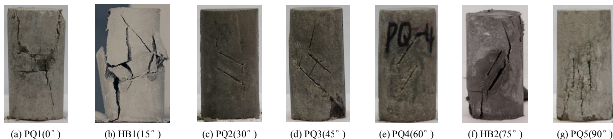
图 9 平行双裂隙岩体破坏形态 Fig.9 Failure modes of specimens with two parallel cracks
