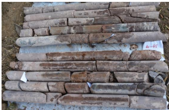
图3 BK21 钻孔 31.3~55.2 m 段整体块石 (“假基岩”) Fig.3 Complete core segment between 31.3 and 55.2 m of borehole BK21
