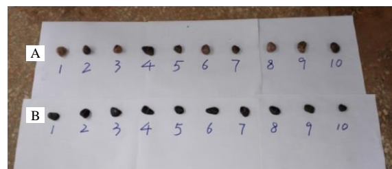
图 2 粒径为 10~20 mm 的部分粗粒料蜡封后照片 Fig.2 Coarse granules between 10~20 mm after wax-coated
