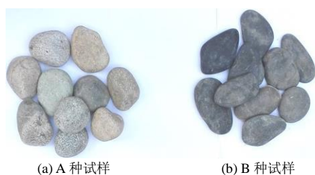
图 1 两种不同外形特征的砂卵石粗颗粒 Fig.1 Two types of coarse granules with different appearance characteristics
