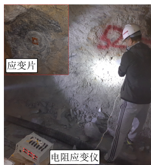
图 6 采用表面应力解除法现场实测洞壁二次应力 Fig.6 Surface stress relief method measuring in-situ secondary wall stress
